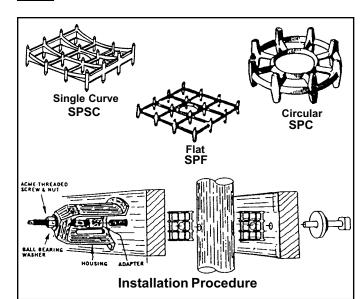
**Spike Grids** are used primarily in pole construction, docks, piling, wharves, and railroad and highway bridges or trestles. Flat and circular grids are used between sawn timbers, while single curve grids are used between round piles or poles and sawn members.
